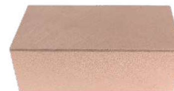
12209 - BLOCK FOR BIOMECHANICAL TESTS 15 PCF WITH BICORTICAL 1MM - 9,5 X 4,5 X 3,2 CM
