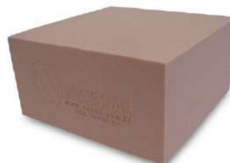
15PCF-CP - BLOCK FOR BIOMECHANICAL TESTS - L 9,7 X C 10 X A 5 CM - 15 PCF
