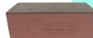
15PCF-CP1 - BLOCK FOR BIOMECHANICAL TESTS WITH CORTICAL 1MM - L 4,5 X C 9,5 X A 3,1 CM
