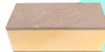
12208 - BLOCK FOR BIOMECHANICAL TESTS 20 PCF WITH BICORTICAL 3MM - 9,5 X 4,5 X 3,6 CM
