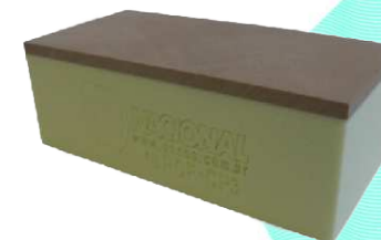
10PCF-CP3 - BLOCK FOR BIOMECHANICAL TESTS WITH CORTICAL 3MM - L 4,5 X C 9,5 X A 3,3 CM
