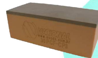
30PCF-CP3 - BLOCK FOR BIOMECHANICAL TESTS WITH CORTICAL 3MM - L 4,5 X C 9,5 X A 3,3 CM
